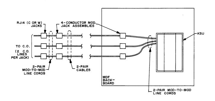
FIGURE 3-6. MODULAR JACK ASSEMBLY WIRING FOR CO LINES
