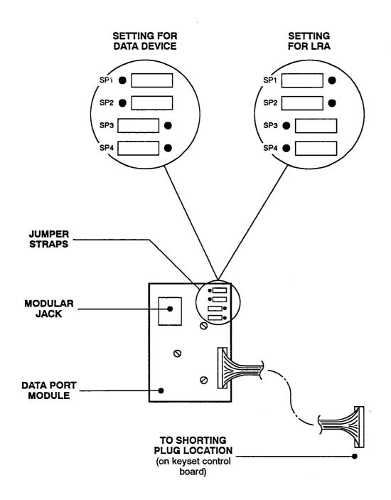
7.14 To connect a Loud Ringing Adapter (LRA): The optional Data Port Module on GLX-Plus Keysets and the ancillary jack (labeled DATA) on Executive Keysets can be used to connect external signaling equipment such as loud bells, horns, flashing lights, etc. to a keyset. This application is useful in areas where the normal ring tone of the keyset cannot be heard, such as warehouses and loading docks. The signaling device follows the normal ringing patterns of the keyset.
