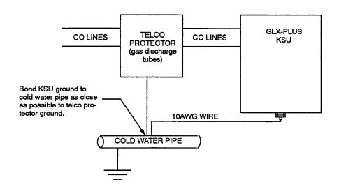
6.7 If the KSU and telco protector are separated by more than 30 feet or if the telco protector ground is inaccessible, additional protection for the C.O. line pairs is recommended. Use a Cook gas protector (part number 502A1-2-LCGX for 2-line, 502A1-4-LCGX for 4-line, 502A1-6-LCGX for 6-line) or equivalent and connect a 10AWG wire between the KSU grounding lug
