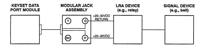
NOTE: Each time the keyset rings, the Data Port Module provides 20-26mA of loop current to the LRA. This causes the LRA contacts to close and activates the signaling device. The LRA is not affected by the ring tone or the ringer volume of the keyset. The LRA must be capable of operating on 20mA current (approximately 20VDC).
